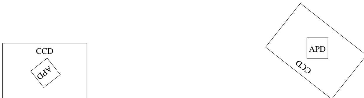
Figure 7: Orientations of the APD in the CCD frame, and of the CCD in the APD frame. The text is oriented appropriately, so that it would be legible with no rotations or reflections on the display of each device.
