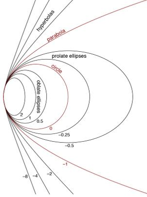
Figure 1: Various forms of conic section as a function of the conic constant,  $K$ .
