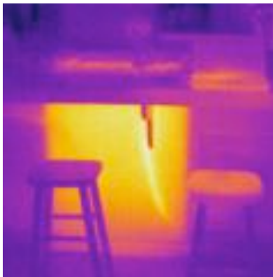
FIGURE 2. Example infrared view of a dishwasher in action. The dishwasher is situated within a counter-top “peninsula,” so that this view is of the back side, covered by thin wood paneling. Note the hot water supply line, the warmed counter-top, the laptop on the counter at right, and that one of the two stools has recently been sat on. The temperature range in this image runs from about 22°C to 35°C.
