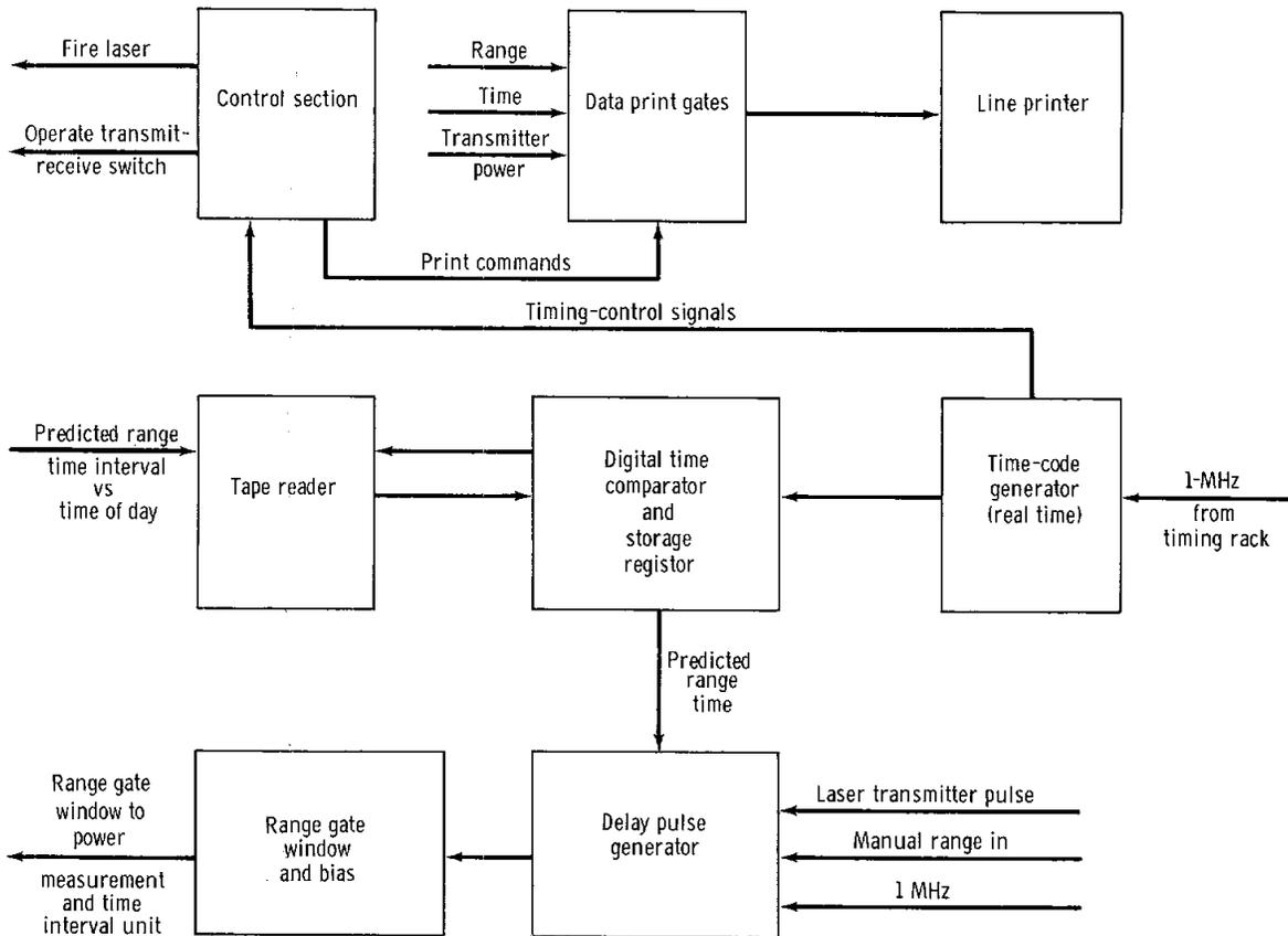
FIGURE 7-19. — Range gate generator and data control.
