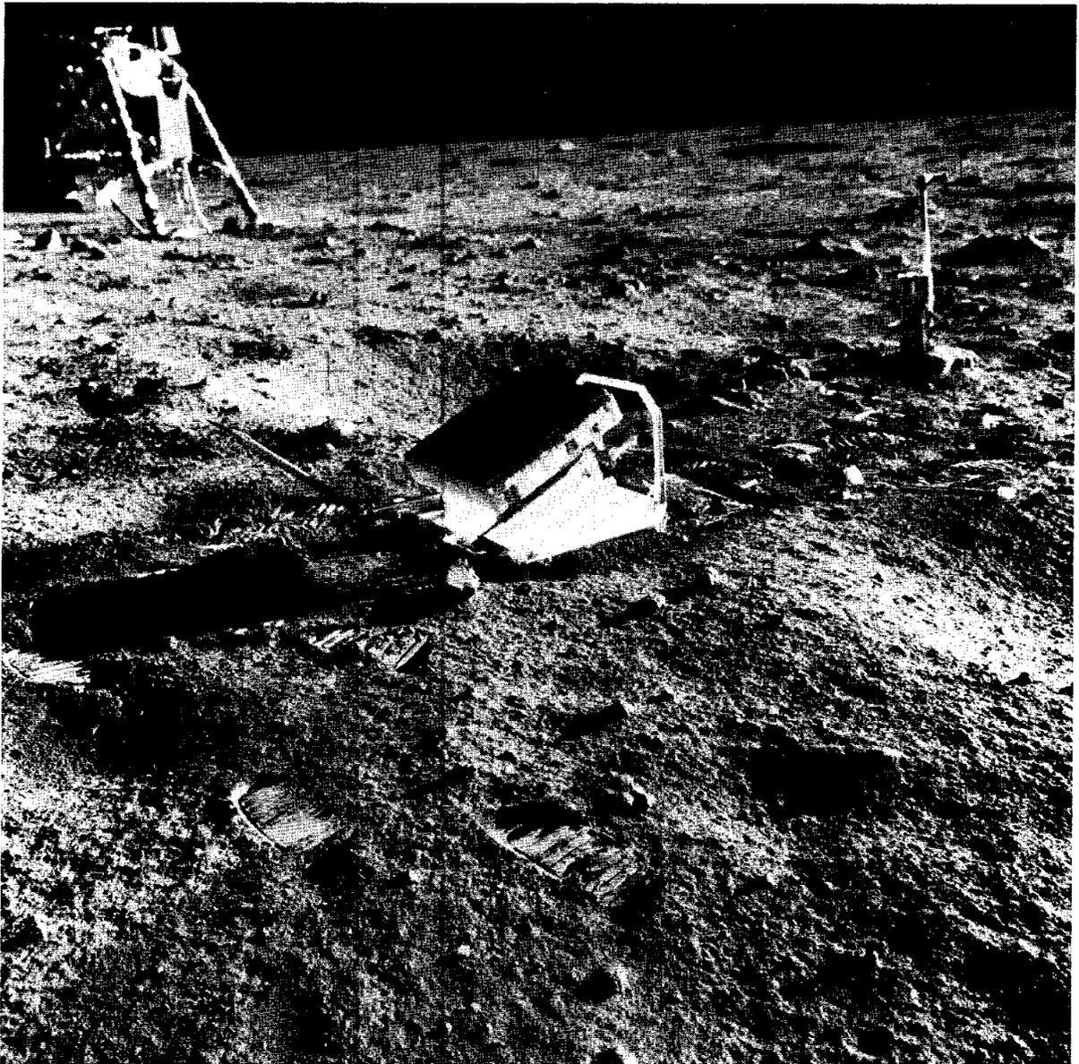
FIGURE 7-7. — The LRRR deployed on the Moon.
