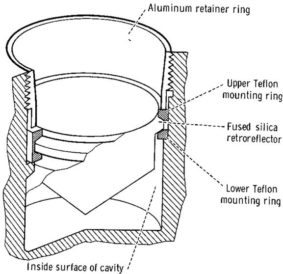
FIGURE 7-1. - Corner reflector mounting.
