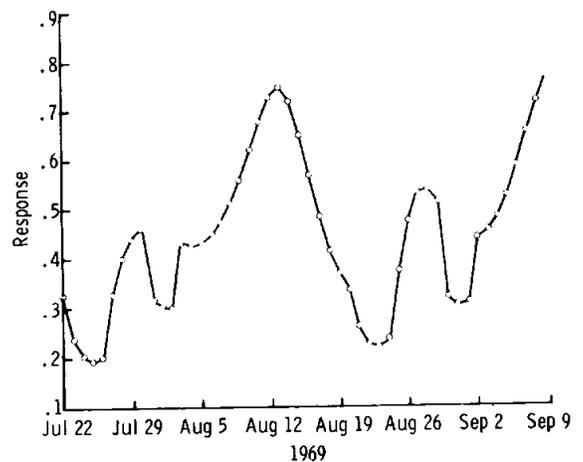
FIGURE 7-5. — Upper bound of LRRR efficiency as a function of time.
