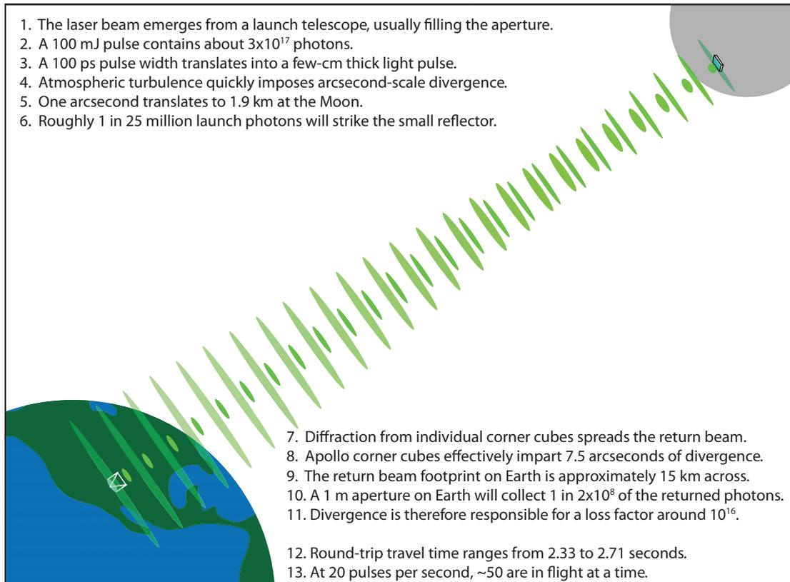
**Figure 2.** Cartoon schematic of LLR technique and divergence-related challenges.
