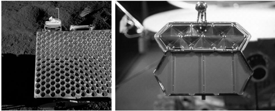
**Figure 4.** A portion of the Apollo 15 reflector (left; courtesy NASA), consisting of 300 corner cube reflectors each 3.8 cm in diameter. All Apollo reflectors are mounted in a similar aluminum tray, except that the Apollo 11 and Apollo 14 reflectors are 100-element arrays arranged in a 10×10 square pattern. At right is the Lunokhod reflector design (courtesy the Lavochkin Association).
