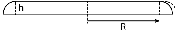
Figure 2: Geometry for overflow atop the cup. We investigate what keeps the bulge from pushing out to the side.
